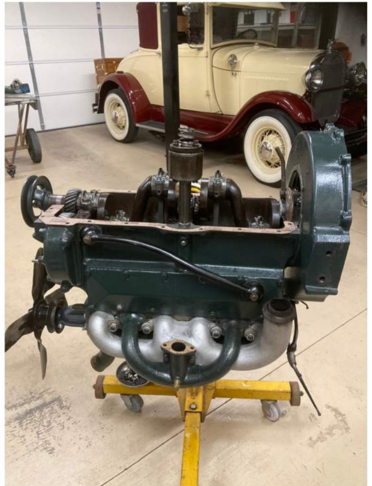
Re-shimming rods are going back together. Will be putting on test stand and running before installing.
